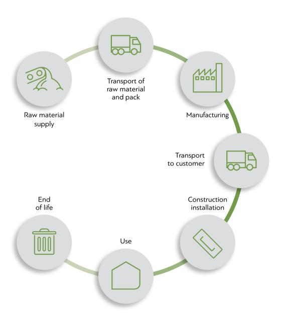
**Declared unit:** The declared unit covers 1m<sup>2</sup> of external thermal insulation composition systems (ETICS) with an insulation layer of 7 cm as installed over a reference service life of 50 years.
