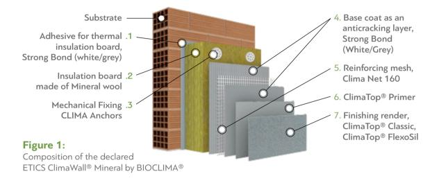
The ETICS consists of several layer, starting from the substrate/masonry:
