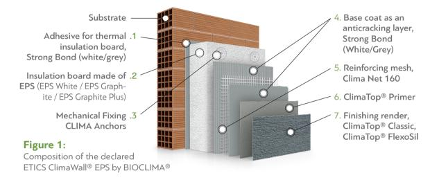
The ETICS consists of several layer, starting from the substrate/masonry:
